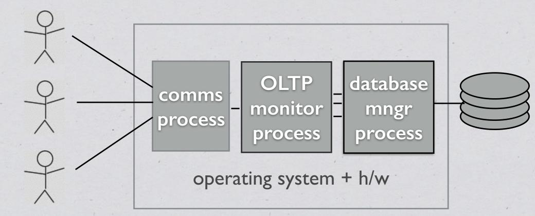
Comms process owns network; application segments run on one monitor thread per user; they share "access ports" to database manager process, which owns data resources
