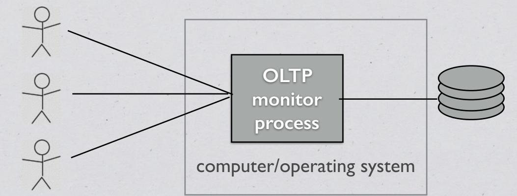
One OS "process" does all the work of managing terminals and data accesses; application segments run on a monitor "thread" for each user but own no resources
